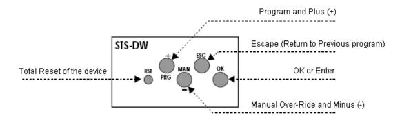
All functions of the time switch are controlled by these 4 buttons. Each button has 2 methods of control used when selecting different options when programming the time switch. Each button can be pressed for <1s (short press) or >1s (long press). The PRG Button is also used as a + Plus and the MAN button is used as a – Minus.
