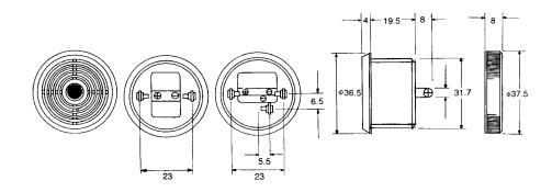
**Connections:** 0.8 x 4.76 tinned brass `male push' on terminal tapped for screw fixing. Two zinc plated steel screws are fitted. Terminal marked + and - on all models.
