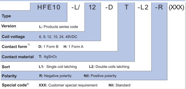
Notes: 1) H means that relay is on the "reset" status when delivery; D means that relay is on the "set" status when delivery. If no speical required by customer, we will keep the relay on the "set" status when delivery.
