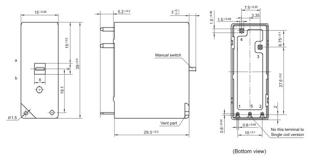
Remark: When the manual switch is pitched on point a, the contact is open; when the manual switch is pitched on point b, the contact is closed.
