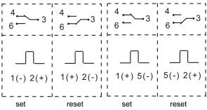
Single coil latching, 1 Form B Double coils latching, 1 FormB
