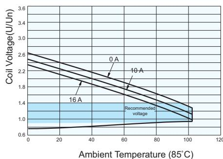
**Notes:** \* The use of a relay with an energising voltage other than the rated coil voltage may lead to reduced electrical life.
