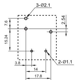
Remark: 1) In case of no tolerance shown in outline dimension: outline dimension  $\leq 1$ mm, tolerance should be  $\pm 0.2$ mm; outline dimension  $> 1$ mm and  $\leq 5$ mm, tolerance should be  $\pm 0.3$ mm; outline dimension  $> 5$ mm, tolerance should be  $\pm 0.4$ mm.
